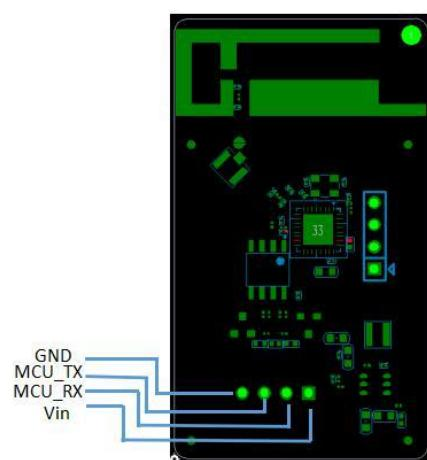
2) Module placement on the motherboard (see below): 1, the recommended antenna part beyond the motherboard edge ; 2, antenna part PCB hollowed;
