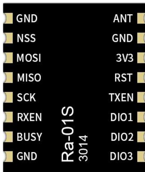
Ra-01SC Pin diagram
