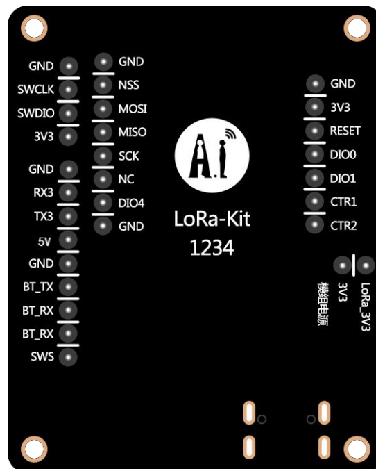
Figure 10 Schematic diagram of pin
