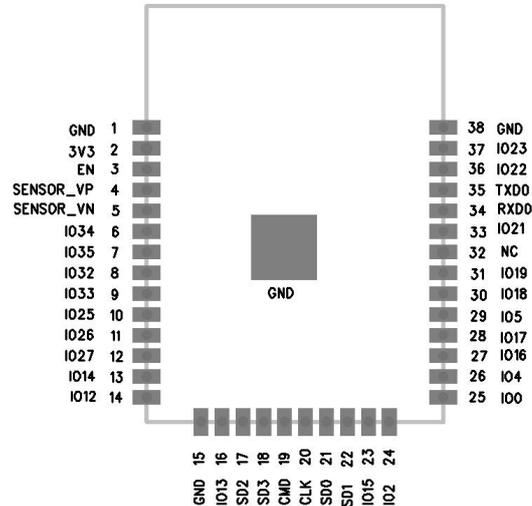
ESP32-SL PIN definition diagram
